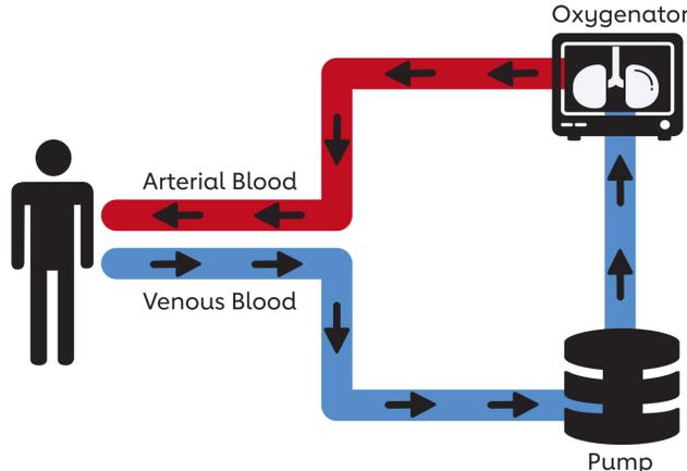
Extracorporeal CPR is performed with an **extracorporeal membrane oxygenation device**. It includes a venous cannula, a pump, an oxygenator, and an arterial cannula.
